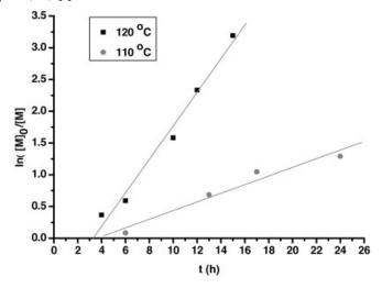
**Figure 5.** Kinetic plots of the bulk ATRP of St at 110 and 120  $^{\circ}$ C. Polymerization conditions: [St]<sub>o</sub>/[BDCIB]<sub>o</sub>/[CuBr]<sub>o</sub>/[PMDETA]<sub>o</sub> = 100:1:0.5:1.5.
