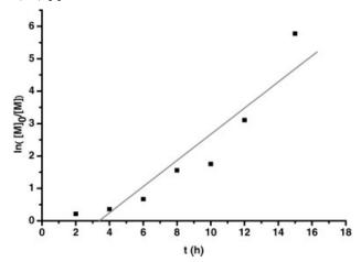
**Figure 7.**Kinetic plot of the bulk ATRP of St at 115 °C. Polymerization conditions: [St]<sub>o</sub>/[TDCIB]<sub>o</sub>/[CuBr]<sub>o</sub>/[PMDETA]<sub>o</sub> = 100:1:1:3.
