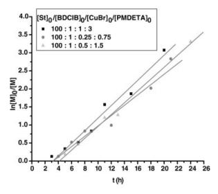
Figure 1. Kinetic plots of the bulk ATRP of St at 115 °C. Polymerization conditions:  $[St]_o/[BDCIB]_o/[CuBr]_o/[PMDETA]_o = 100:1: n: 3n (n = 1, 0.50, .25).$
