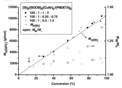
Figure 2. Dependence of  $M_{n(GPC)}$  and  $M_w/M_n$  on the monomer conversion for the bulk ATRP of St. Polymerization conditions are same as in Figure 1.
