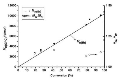
**Figure 8.** Dependence of  $M_{n(GPC)}$  and  $M_w/M_n$  on the monomer conversion for the bulk ATRP of St. Polymerization conditions are same as in Figure 7.
