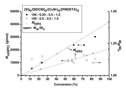
**Figure 4.** Dependence of  $M_{n(GPC)}$  and  $M_w/M_n$  on the monomer conversion for the bulk ATRP of St. Polymerization conditions are same as in Figure 3.
