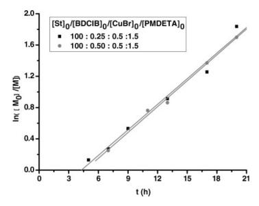
Figure 3. Kinetic plots of the bulk ATRP of St at 115 °C. Polymerization conditions:  $[St]_o/[BDCIB]_o/[CuBr]_o/[PMDETA]_o = 100$ : n: 0.5:1.5 (n = 0.25, 0.50).
