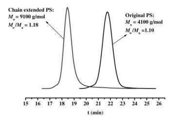
Figure 10. GPC curves of original PS and chain extended PS. Chain extension conditions via ATRP:  $[St]_0/[Macroinitiator]_0/[CuBr]_0/[PMDETA]_0 = 100:1:1:3, St/DMF = 1:1 (v/v), 115 °C, 13 h, conversion(%) = 40.7%.$
