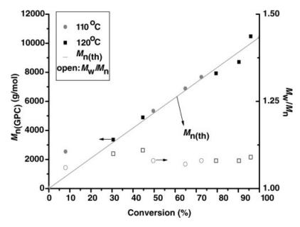
**Figure 6.** Dependence of  $M_{n(GPC)}$  and  $M_w/M_n$  on the monomer conversion for the bulk ATRP of St. Polymerization conditions are same as in Figure 5.
