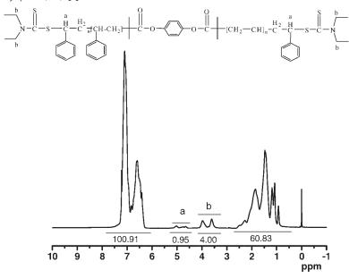
**Figure 9.** 400 MHz  $^1$ H NMR spectrum of the PS prepared using BDCIB/CuBr/PMDETA system in bulk ([St] $_o$ /[BDBB] $_o$ /[CuBr] $_o$ /[PMDETA] $_o$  = 100:1:1:3) at 115  $^\circ$ C (CDCl $_3$ ). Sample:  $M_{n(GPC)}$  = 4100 g  $\cdot$  mol  $^{-1}$ ,  $M_w/M_n$  = 1.10.
